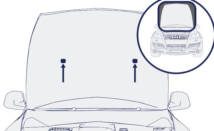
Use "plastic clips of bonnet insulation" or holes to attach the PA2 AUTOMOTIVE fire extinguishing system.
