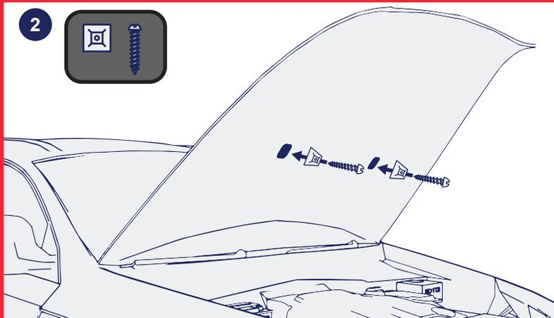
Screw the enclosed plastic squares into the "plastic clips of bonnet insulation".
