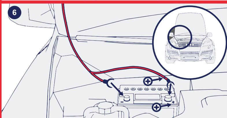
In the last step, connect the wires to the car battery (red plus to plus and blue minus to minus)
