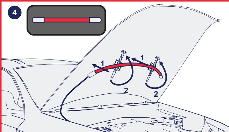
Then place the fire extinguishing system in a pre-selected location and tighten appropriately with the "zip ties".
